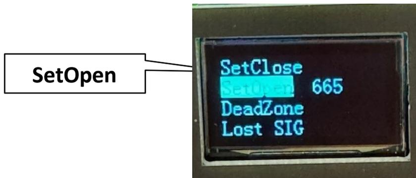
12. Select the OPEN position by increasing or decreasing the resistance value (in ohms) using the UP and DO buttons to select the appropriate value once the valve is exactly open.
