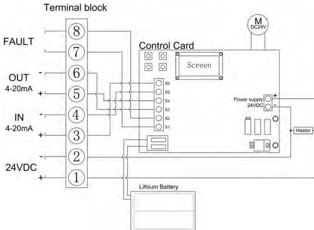
**VTM Modulating Version 1.0 with Battery Backup Wiring Diagram (120VAC)**
