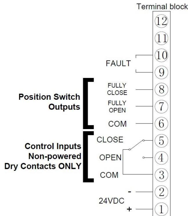
**VTM On-Off Version 1.0 with Battery Backup Wiring Diagram (120VAC)**
